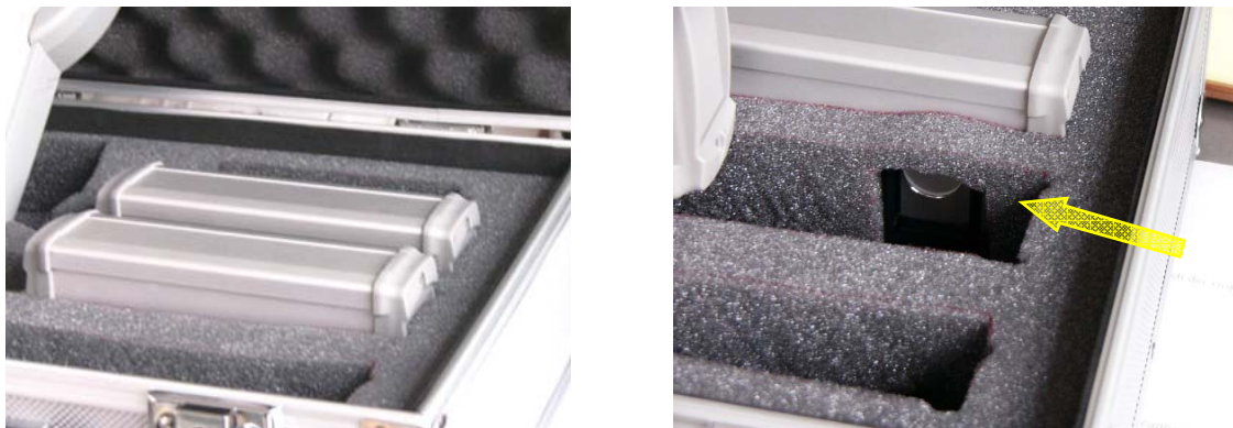
Figure 5: Left, the sender and receiver in their safety place in the case. Right, the arrow depicts where to place the 70% filter.
